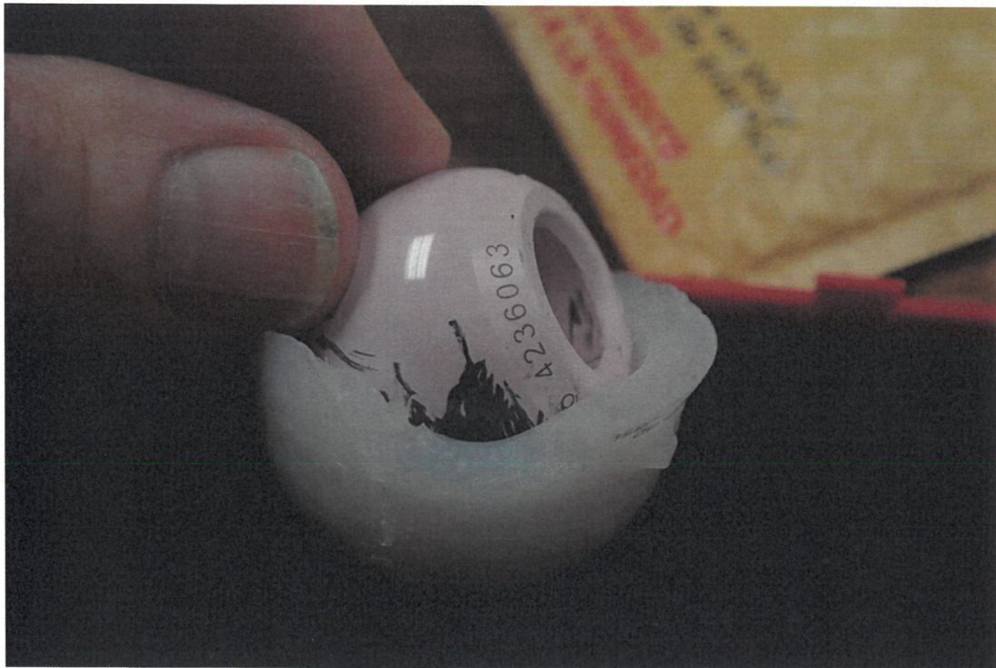
Figure 9 Stem angle matching the deformation of the remaining lip portion
