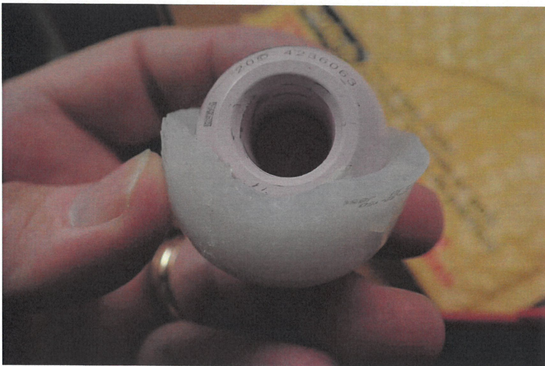
Figure 8 Head in the liner showing the conformance of the stem to the divot in the liner lip
