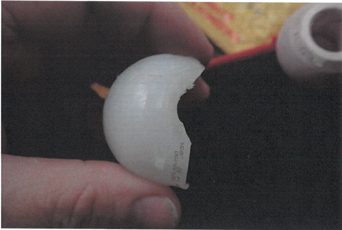
Figure 7 Equatorial view of the damaged liner
